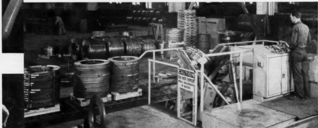
Operator selects number of straps and strap position for coils of various sizes. Here, coils are also automatically stacked on pallets and up-ended for lift truck handling.
